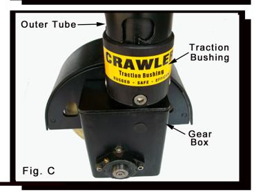
**NOTE:** With the traction bushing installed, a portion of the weight from the scaffold and the operator is now transferred to the drive wheel, therefore increasing the traction.
